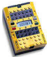
Fig. 1. The RCX, the “heart” of a Mindstorms robot
